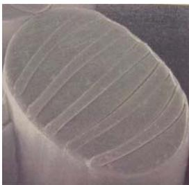
WRAMP fiber is a bicomponent fiber with a stacked structure consisting of eleven alternating layers or “stripes” of polyester and nylon. Mild refining of this fiber causes it to split into approximately 0.3 micro denier ribbon shaped fibers. Papers made from WRAMP fiber, or blends with wood pulp, exhibit very high tear factor, low air permeability, smaller pore size, high luster, good printability and high fold endurance.
